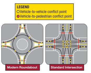
Figure 4.9: Vehicle-vehicle and vehicle-pedestrian conflict points
