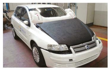
Figure 5.2: Test vehicle with pedestrian air bag and advanced vehicle design (Photo copyright and re-printed with the express permission of Fiat Research Center: an APROSYS research project sponsored by the European Commission: www.aprosys.com)
