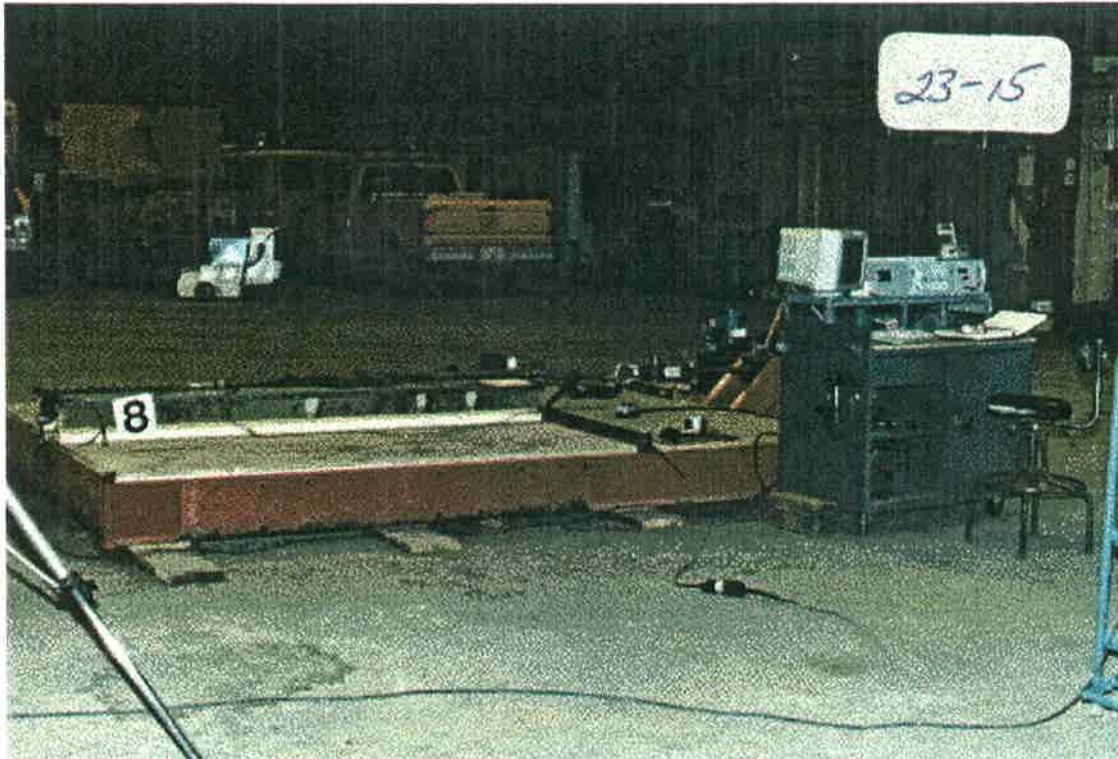
Figure 1/ Test rig, with 2.44 m (8 ft) wide plate, set for a lateral pull
