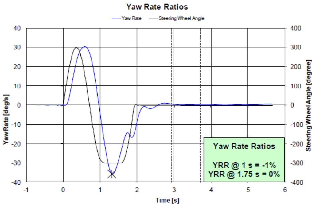
To comply with CMVSS 126, the ESC system must meet various requirements; in particular, when the vehicle undergoes Sine with Dwell manoeuvres, the yaw rate ratio must be smaller than
