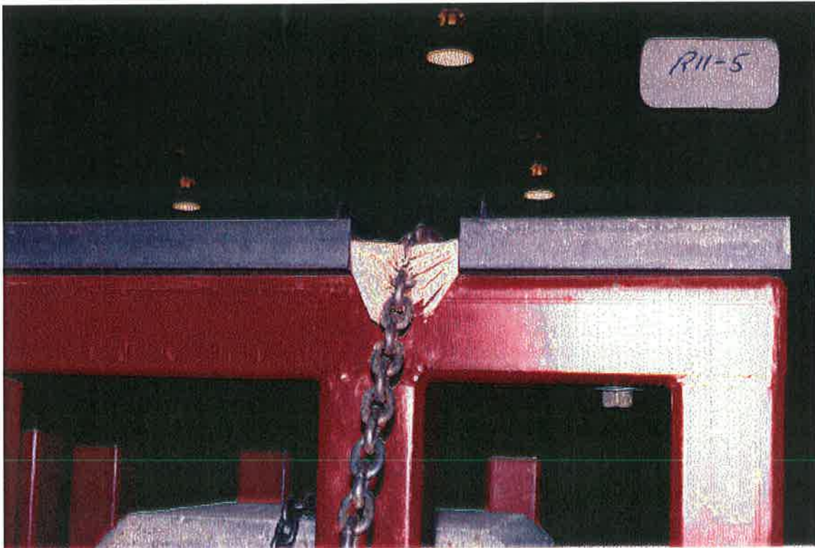
Figure 9/ Wood Corner Damaged by Chain after Lateral Pull
