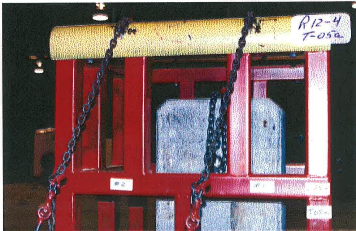
Figure 14/ Chain Tiedowns Move with Carriage during Longitudinal Pull
