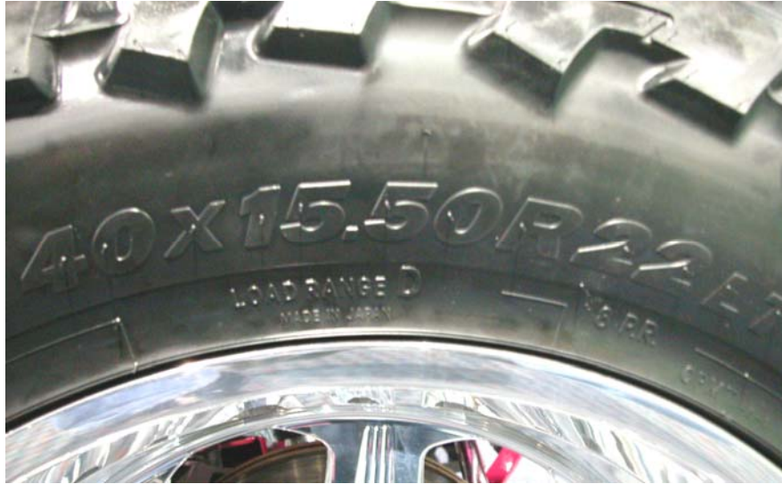
Figure 6 - Illustration of Sidewall Markings on a Tire Used in Raised Vehicle Applications
