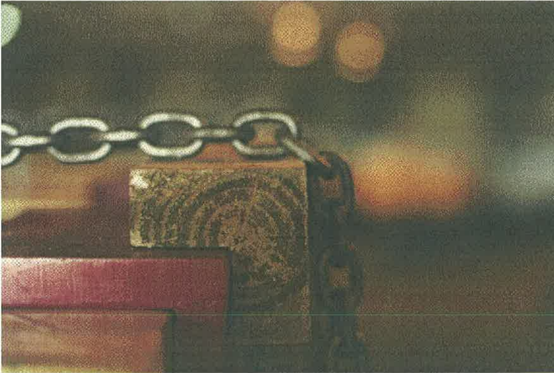
Figure 9/ Square Wood Corner with Chain Tiedown
