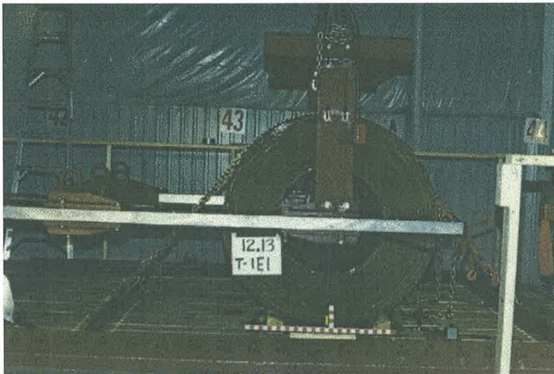
Figure 41/ Lateral pull with chain tied down over coil in a cradle
