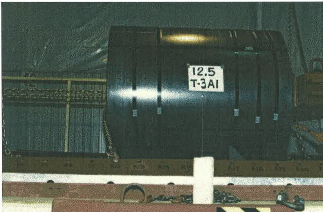
Figure 27/ Setup after longitudinal pull with chain securement 10,523 kg (23,200 lb) coil with two 3/8 in chains at 85/-85 deg
