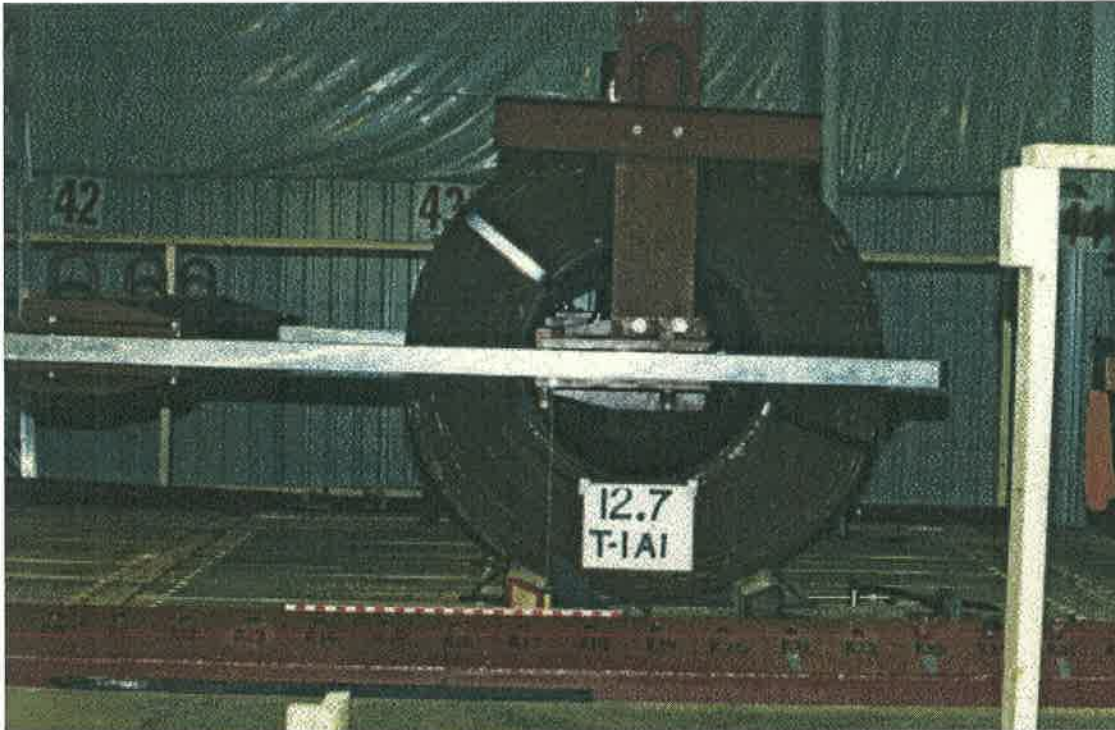
Figure 29/ Setup for friction of cradle Lateral pull for 10,523 kg (23,200 lb) coil
