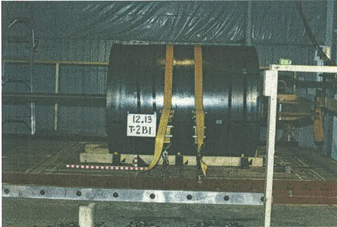
Figure 40/ Longitudinal pull with webbing tied down over coil in a cradle
