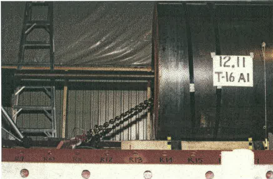
Figure 37/ Setup for longitudinal pull of coil in unsecured cradle 10,523 kg (23,200 lb) coil with 3/8 in chain tiedowns at steep angle
