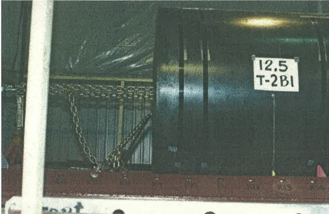
Figure 24/ Setup for longitudinal pull with chain securement 10,523 kg (23,200 lb) coil with two 3/8 in chains
