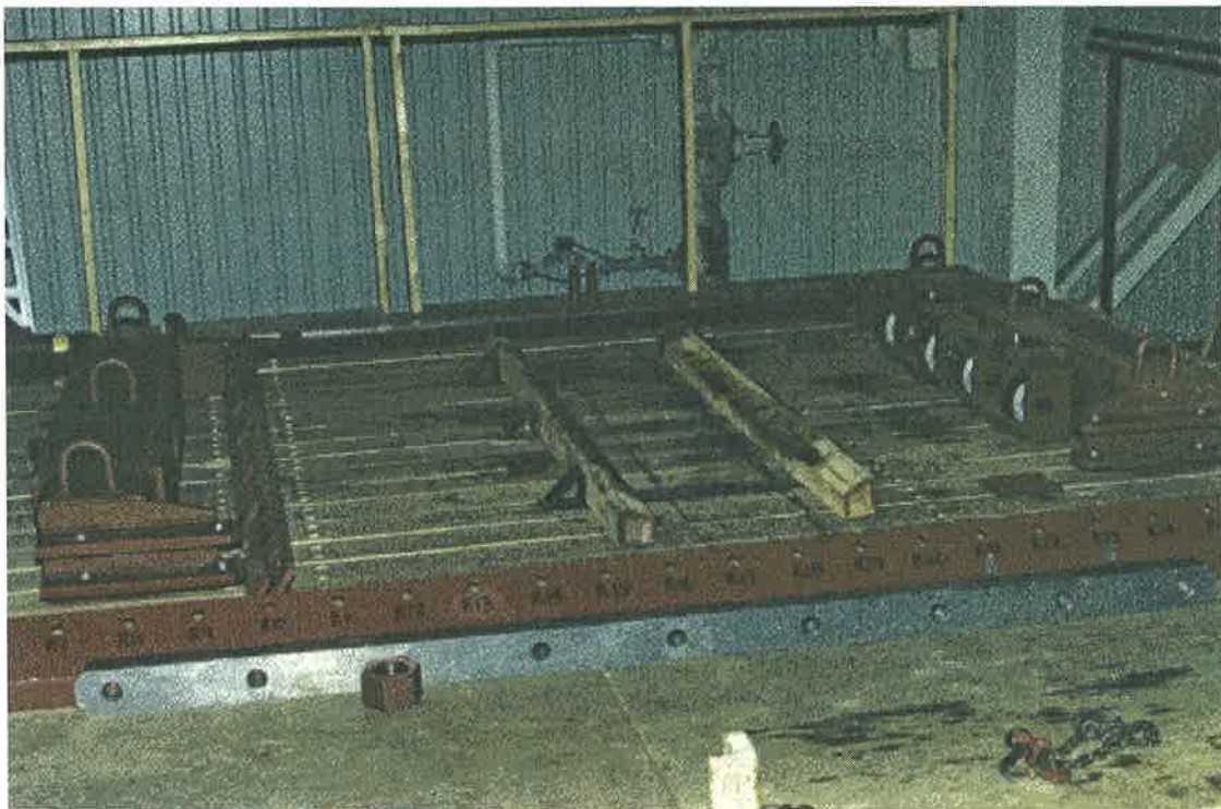
Figure 2/ Deck of test rig, showing side rails, cradle and crossmembers
