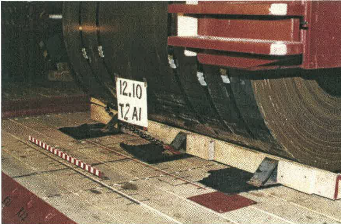
Figure 35/ Setup for friction of coil secured to unsecured cradle Longitudinal pull of 20,139 kg (44,400 lb) cradle on rubber mats
