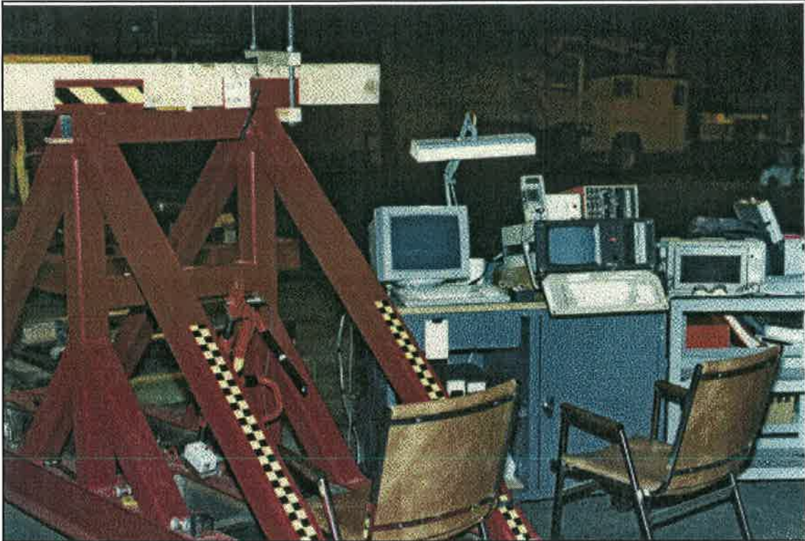
Figure 4/ Dunnage Test Reaction Frame and Data Acquisition Equipment
