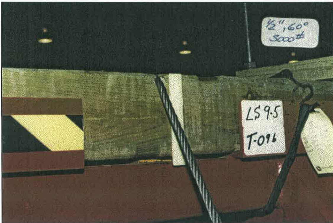
Figure 16/ Damage to Spruce by Wire Rope Tiedown
