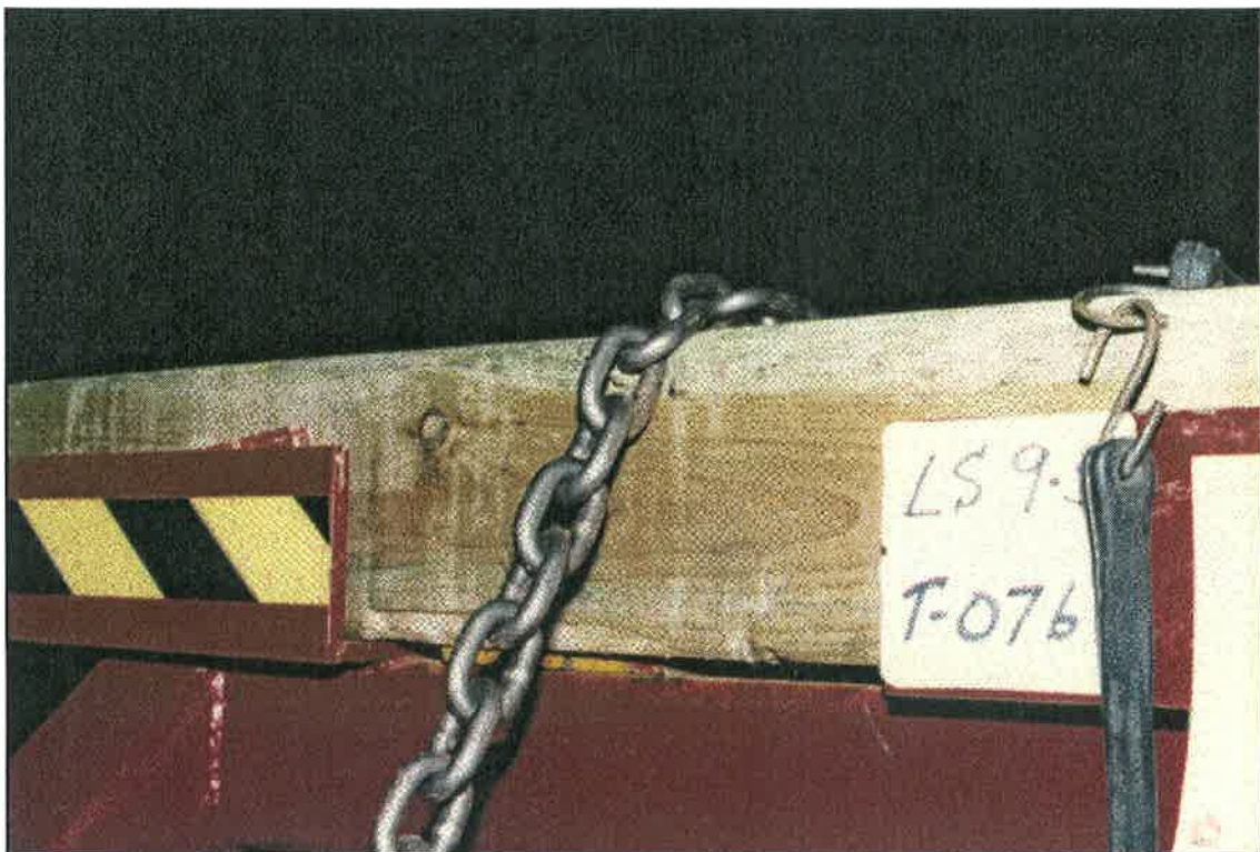
Figure 7/ Chain Tiedown Indenting and Splintering Spruce
