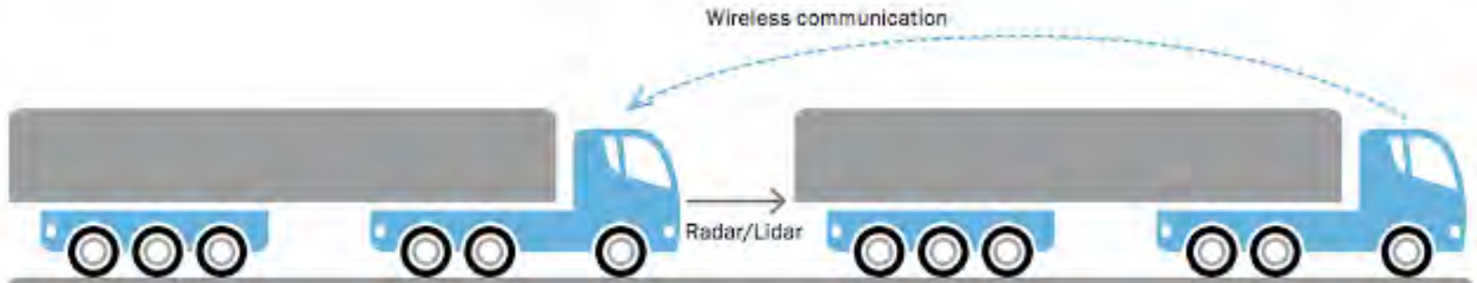
Fig. 2. A two-truck platoon with wireless communication and radar technology
