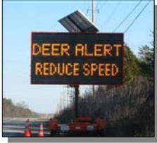
Variable message signs (5) displaying “DEER ALERT - REDUCE SPEED“(in both English and French) were placed along the 20 roadways with high incidents of wildlife collisions. Each board was in place for one week and then moved to the next location.
