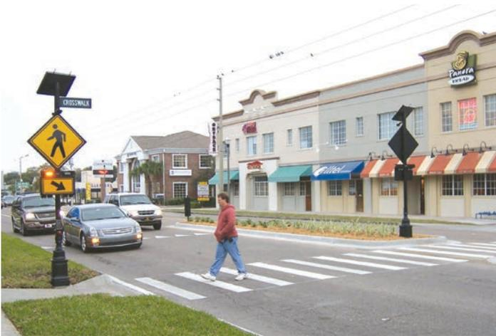
Figure 4.14: Rectangular Rapid-flashing Beacon (RRFBs),
