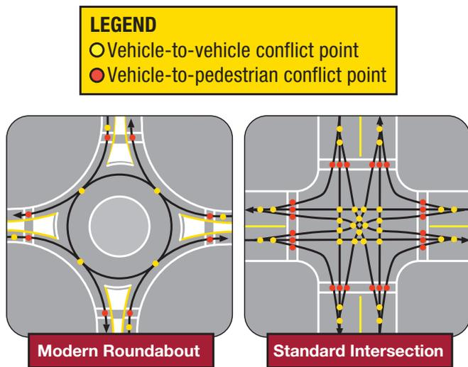
Figure 4.9: Vehicle-vehicle and vehicle-pedestrian conflict points
