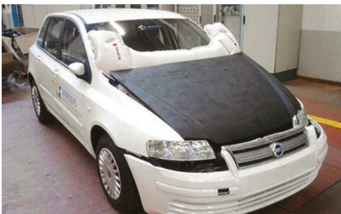
*Figure 5.2: Test vehicle with pedestrian air bag and advanced vehicle design (Photo copyright and re-printed with the express permission of Fiat Research Center: an APROSYS research project sponsored by the European Commission: [www.aprosys.com](http://www.aprosys.com))*
